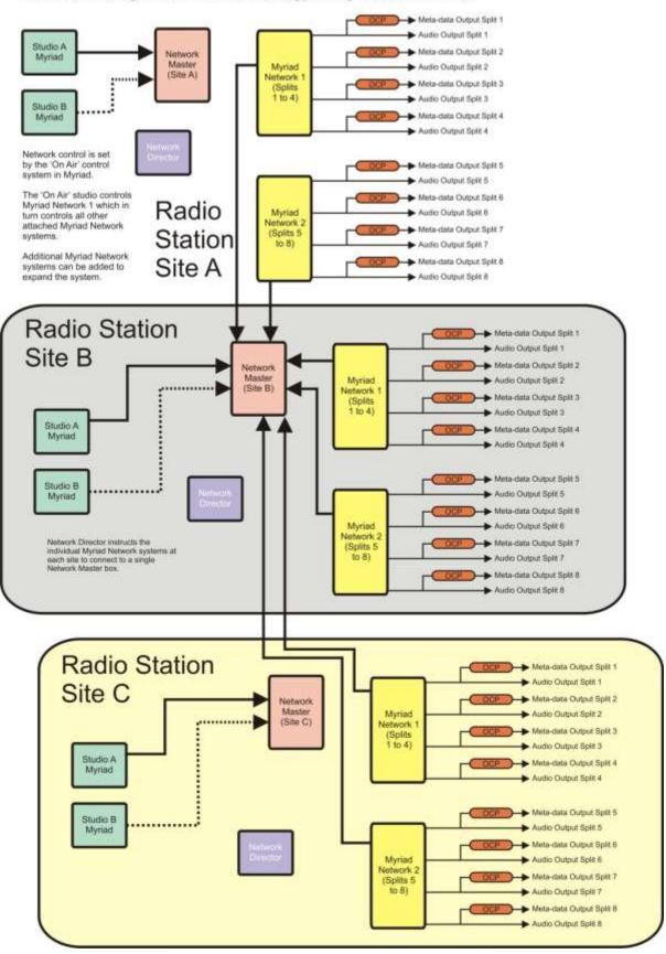
As you can see, this it different to the second scenario we looked at in that the Myriad Networks are connecting directly to the primary Network Master ignoring the local Network Master altogether. This is necessary to allow the remote configuration of the network via Network Director.
